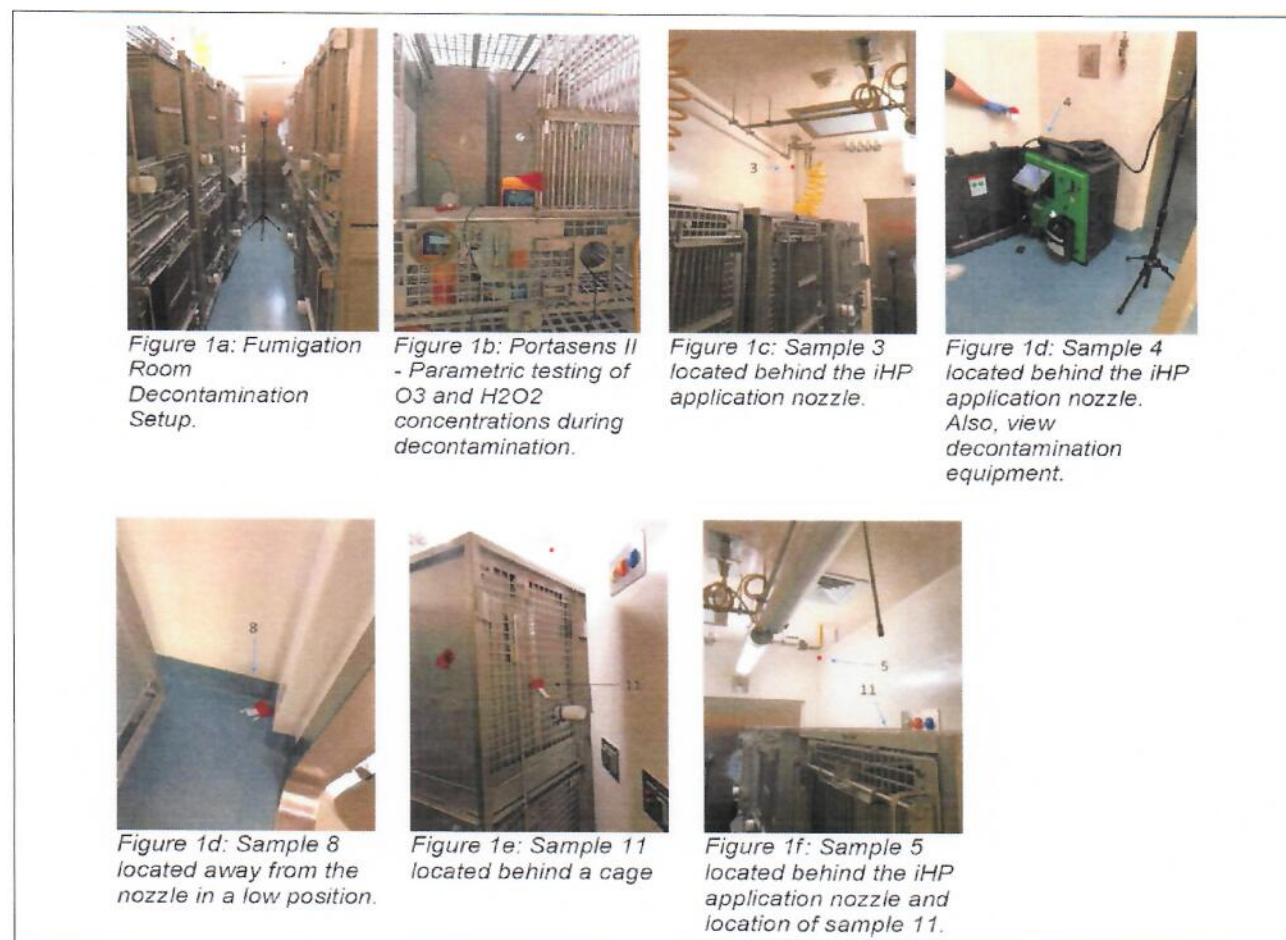
Figure 1. (a) Fumigation room decontamination setup. (b) Portasens II – Parametric testing of O 3 and H 2 O 2 concentrations during decontamination. (c) Sample 3 located behind the ionized hydrogen peroxide (iHP) application nozzle. (d) Sample 4 located behind the iHP application nozzle. Also view decontamination equipment. (e) Sample 8 located away from the nozzle in a low position. (f) Sample 11 located behind a cage. (g) Sample 5 located behind the iHP application nozzle and location of sample 11.
